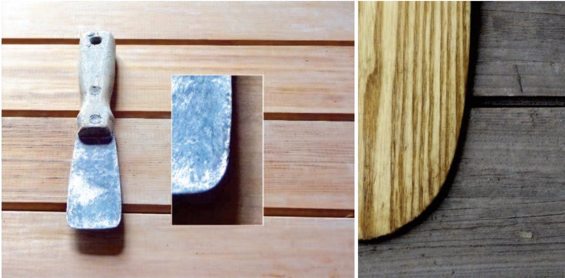
*The once angular corners of a scraper worn into curves by constant use. Such a curve is echoed at the tip of a paddle blade. Such a “pre-worn” shape is more resistant to further abrasion damage.*
